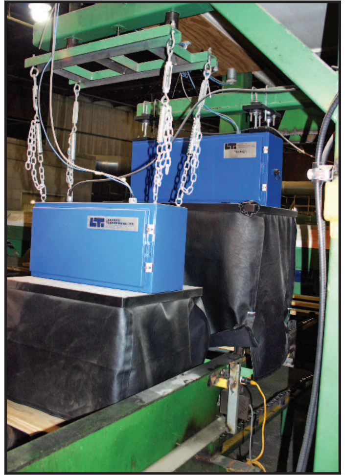
Downstream from grading station, warp scanner, left, and grade mark reader and True-Q system, right, complete planer optimization hardware package.
