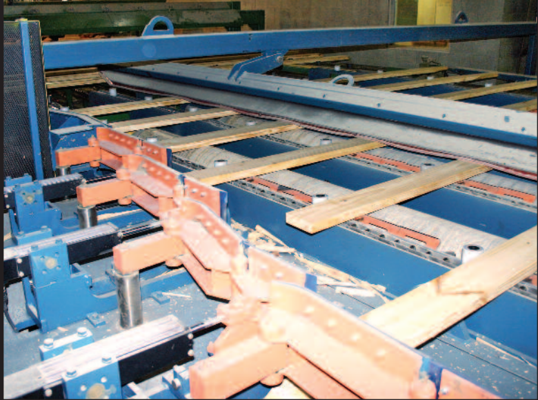
New Comact infinite trimmer fence, left, and Autolog inkjet printer, right, are two components of planer line project.
