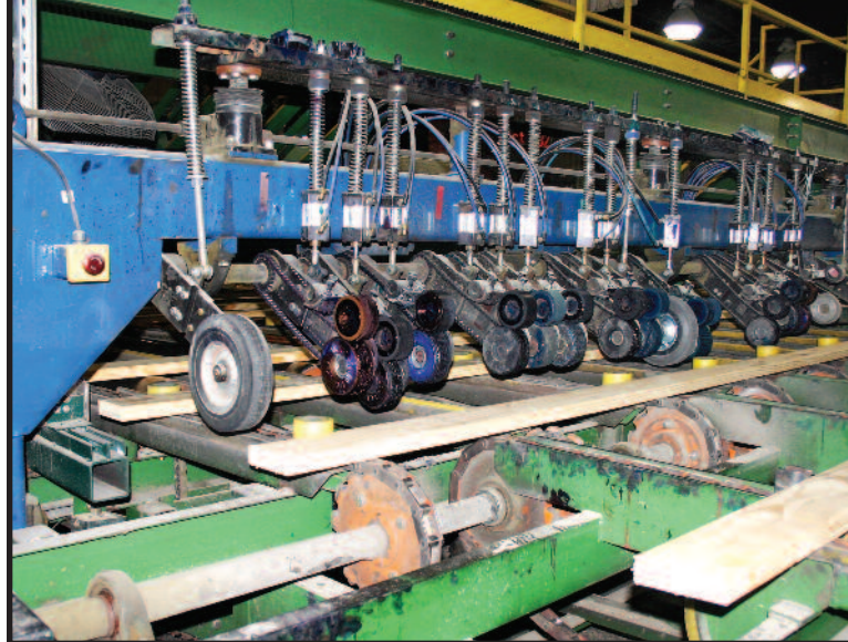
New Comact infinite trimmer fence, left, and Autolog inkjet printer, right, are two components of planer line project.
