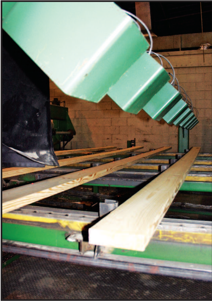
Downstream from grading station, warp scanner, left, and grade mark reader and True-Q system, right, complete planer optimization hardware package.
